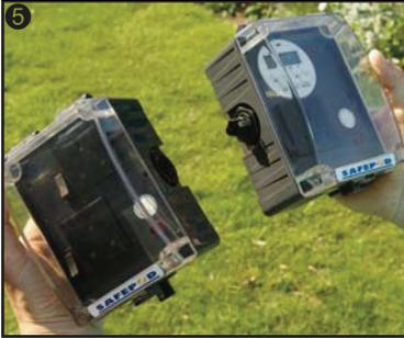
Inserting a flat blade screwdriver into the slot inside the cover can separate the connector on the right hand side of the Safepod module. Disconnect the power before connecting or disconnecting the plugs and sockets.
